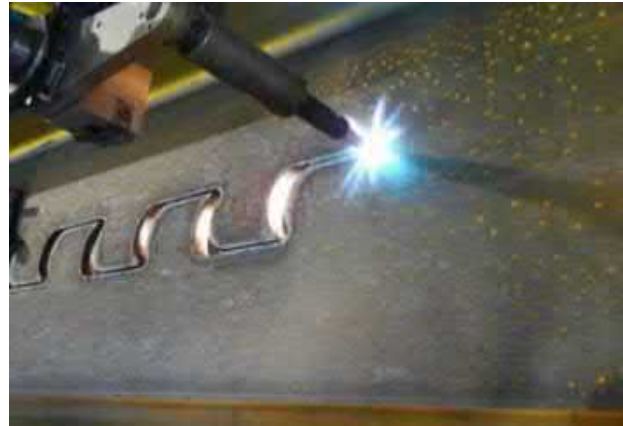
Figure 10: Modification of the SA shape (elimination of sharp notch) [7].
